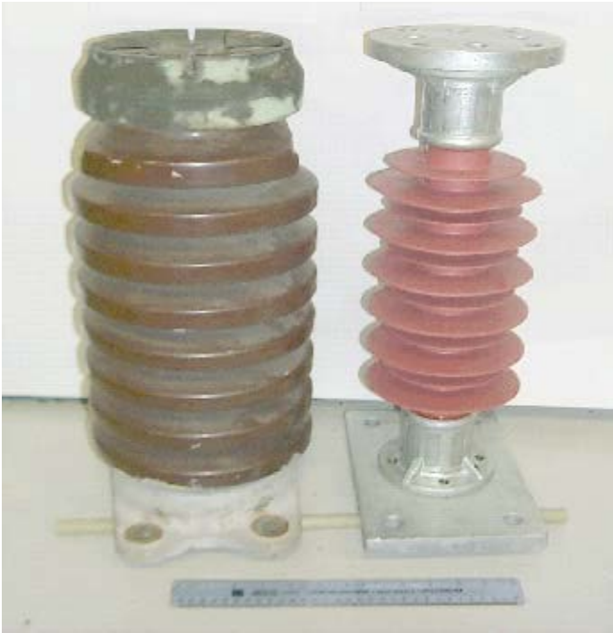
Figure 1. 33Kg vs 16Kg. A26 Porcelain vs. Polymeric. (Source: TE Connectivity)
