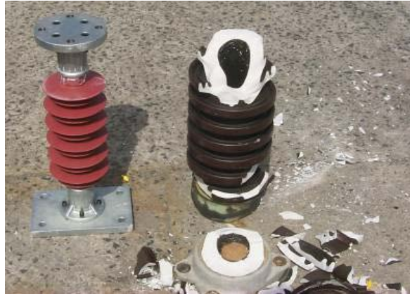
Figure 8a. Damage as a result of drop test. (Source: TE Connectivity)
